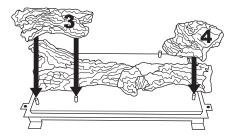
Figure 44 - Installing Logs No. 3 and No. 4
